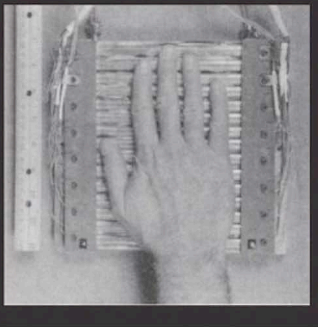
Figure 2: Thunberg's thermal grill is a device the size of one's hand that has alternating independently controlled thermal bars. (5)
