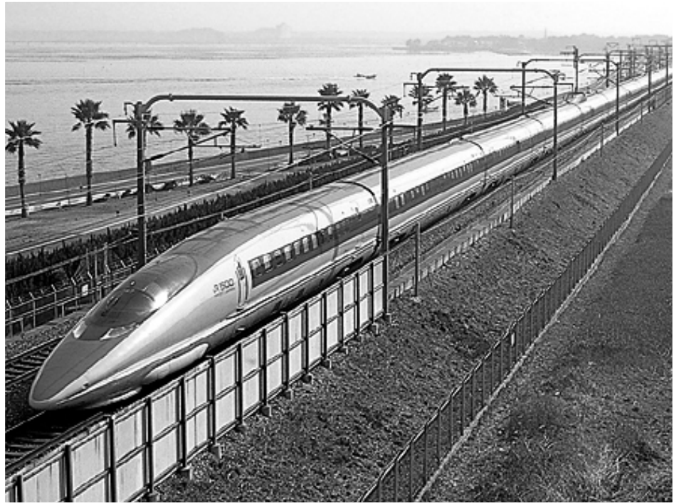
▲ Figure 3. The Shinkansen 500 series, with a nose cone modeled after a Kingfisher, reduced electricity use by 15% compared to the previous model.
